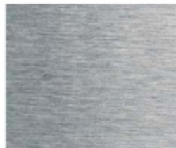
Surface finish: machined, Ra 0.8 \mu m
