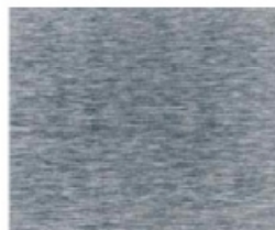
Surface finish: fine-machined, and grinded, Ra 0.2 \mu m
