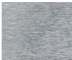
Surface finish: fine-machined, and grinded, Ra 0.4 \mu m
