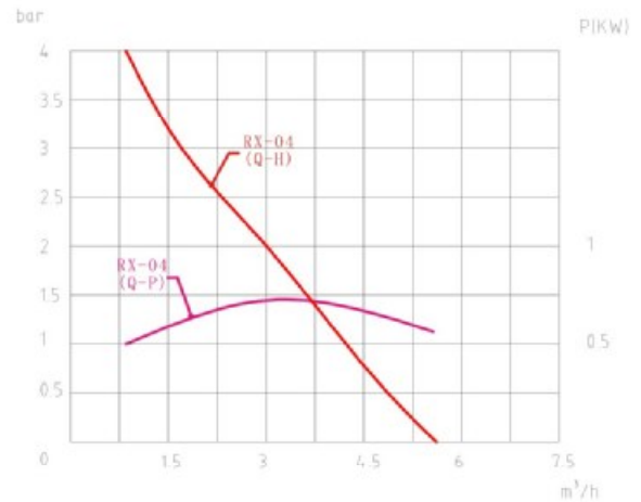
RX-04(带4P电机性能曲线图/Graph) RX-04 Flexible impeller pump (graph for 4P motor performance)
